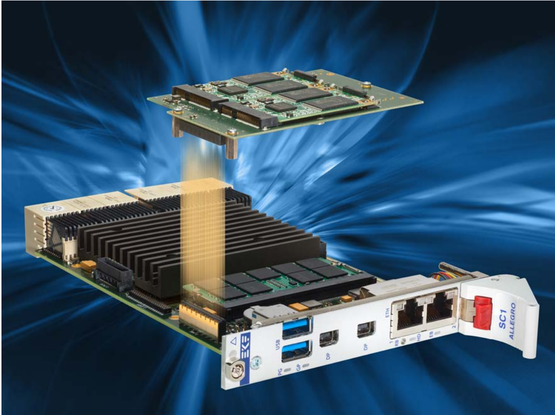
C47-MSATA Mezzanine over CPU Carrier Card
